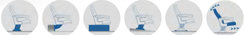
Suelo To the floor Frente Grada Riser-Fixed Sobre Grada On-Steps Pendiente Slope Móvil Movable Seat Sistema Rocker Rocker System
